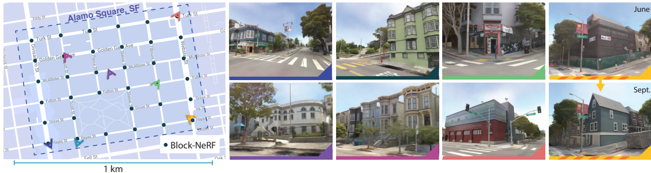
Figure 1. Block-NeRF is a method that enables large-scale scene reconstruction by representing the environment using multiple compact NeRFs that each fit into memory. At inference time, Block-NeRF seamlessly combines renderings of the relevant NeRFs for the given area. In this example, we reconstruct the Alamo Square neighborhood in San Francisco using data collected over 3 months. Block-NeRF can update individual blocks of the environment without retraining on the entire scene, as demonstrated by the construction on the right. Video results can be found on the project website waymo.com/research/block-nerf .
